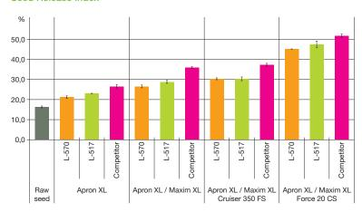
Seed release index (bottom of planter). The lower the value, the higher the accuracy of planting.
